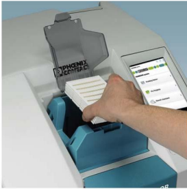
Figure 3-2 Loading sheets to the infeed magazine
